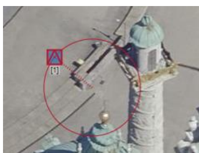
Fig. 12 Display of a measurement contradiction based on an error circle in MEASUREE
