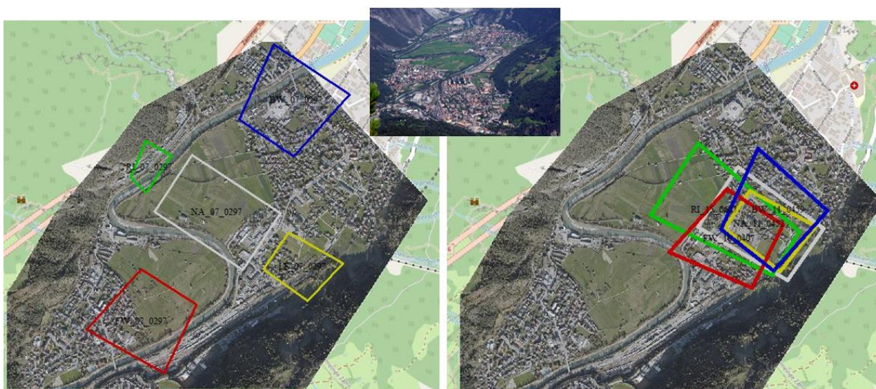
Fig. 3: Footprints of a Maltese Cross camera in the mountains (Zams, Tyrol, 2019). Left = all five images of one trigger point, right = images of all five cameras at one location (different trigger points).
