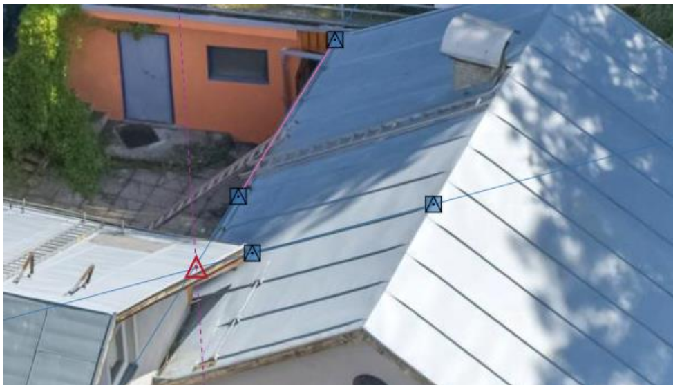
Fig. 19: Guide lines (dashed blue) help with the construction of objects in areas of the image that are difficult to see
