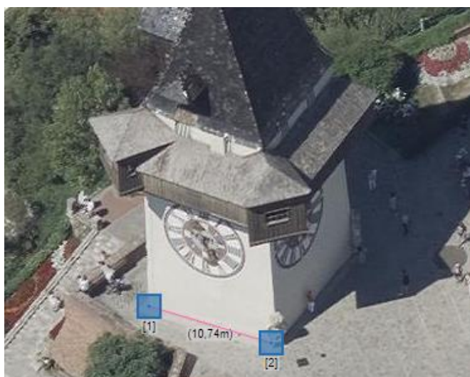
Fig. 17: The distance between point [1] and point [2] is automatically determined and immediately displayed
